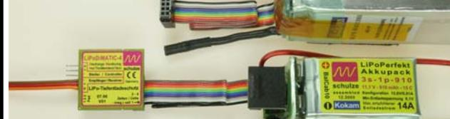
LiPoDiMATIC-SE4 with BalCab10-plug for 2s - 4s packs
