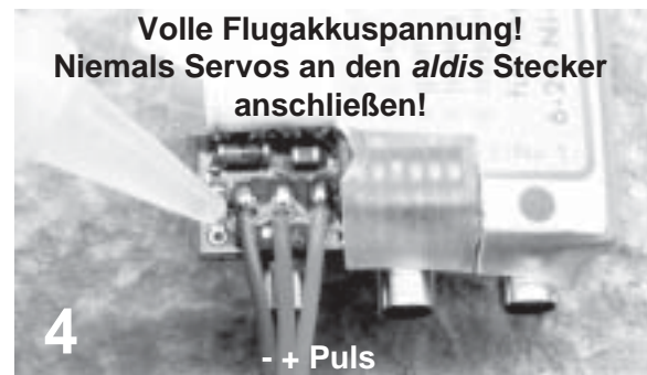
Zugentlastung u. Isolation m. dickflüssigem Sekundenkleber Strain relief and insulation made by thick flowing rapid glue -=braun, +=rot, puls=orange / -=brown, +=red, pulse=orange
